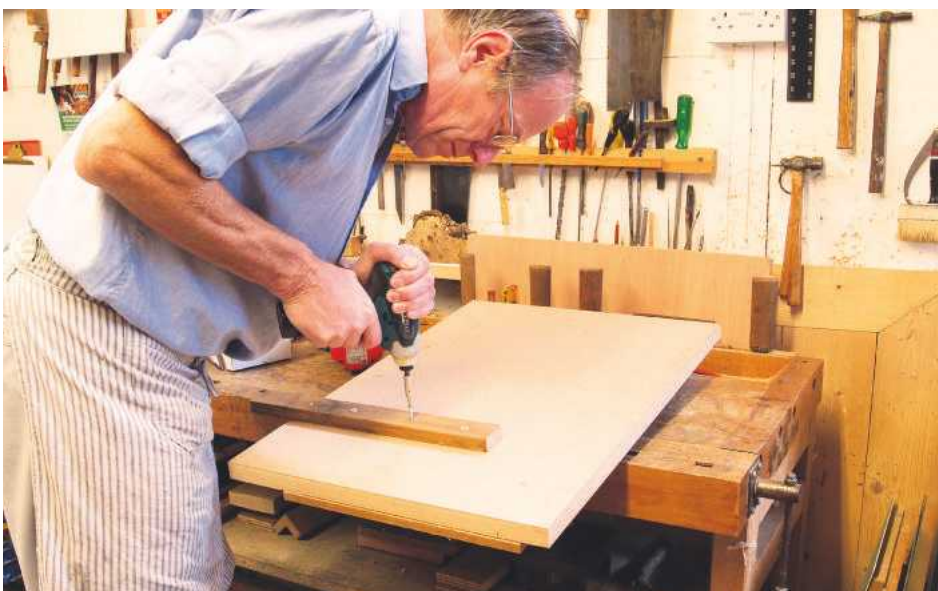
Pic.15 Finally fit a batten to the underside
